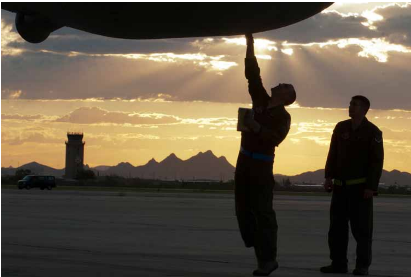
U.S. Air Force Staff Sergeants Thomas Sinon and Chris Bageant, 79th Rescue Squadron flight engineers, pre-flight the refueling pod on a HC-130P Combat King prior to a training mission at Davis-Monthan Air Force Base, Az. on Sept. 23, 2011. The refueling pod houses the hose used to refuel fellow aircraft while in flight. (U.S. Air Force photo by Staff Sgt. Joshua J. Garcia)
