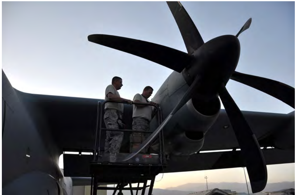
Senior Airman James Mitchell removes an engine cowling on a C-130J Hercules aircraft from the 774th Expeditionary Airlift Squadron here Sept. 20, 2011, as Tech. Sgt. Wayne Warner looks on. Both Airmen are 774 EAS maintainers. Mitchell hails from North Kingston, R.I., while Warner is a native of Warwick, R.I. (U.S. Air Force photo by Staff Sgt. John Wright)
