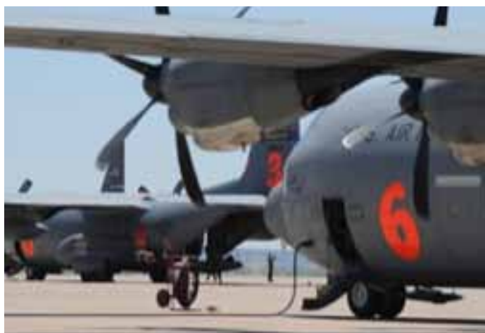
Airmen prepare several C-130 Hercules for wildfire fighting operations across Texas April 18, 2011, at Dyess Air Force Base, Texas. These C-130s are equipped with Modular Airborne Firefighting Systems, which are capable of dispensing 3,000 gallons of water or fire retardant in less than 5 seconds. The wildfires have spread across parts of Texas and have burned more than 1,000 square-miles of land. (U.S. Air Force photo by Tech. Sgt. Robert Wollenberg)
