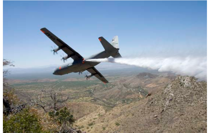
A C-130J from the 146th Airlift Wing based at Point Mugu Naval Air Station, Calif., drops water over the treetops during annual training in South Carolina in April. The unit was the first to transition to the MAFFS 2 system in 2008, and it remains the only unit flying the new system on the C-130J aircraft. (Photo by Airman 1st Class Nicholas Carzis)
