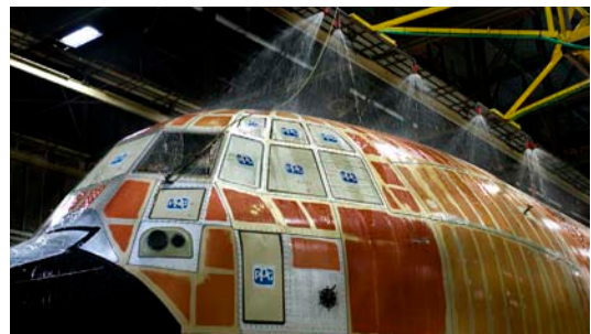
A brand new J undergoes leak testing before heading off to the trim shop.
