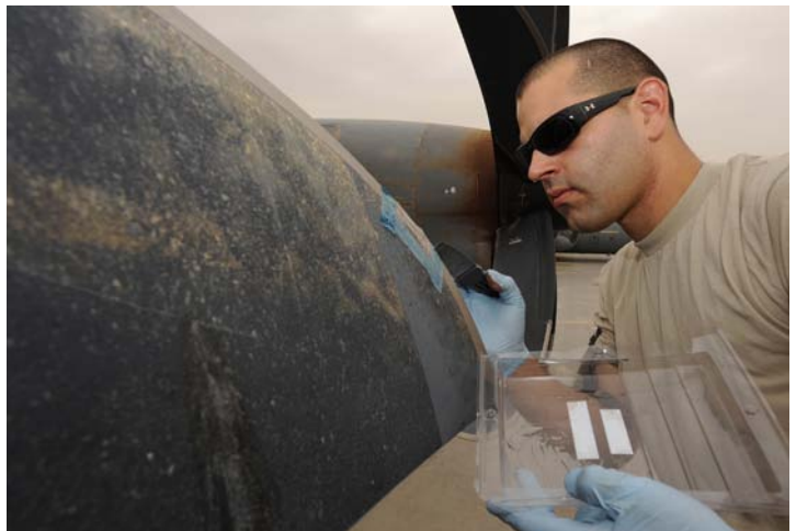
Tech. Sgt. Jeremy Thompson, a 451st Expeditionary Aircraft Maintenance Squadron propulsion systems craftsman, applies a liquid polymer to a C-130J Hercules propeller Aug. 2 at Kandahar Airfield, Afghanistan. Thompson sanded the propeller to the proper contour once the polymer had set. (U.S. Air Force Photo by Tech. Sgt. Chad Chisholm)
