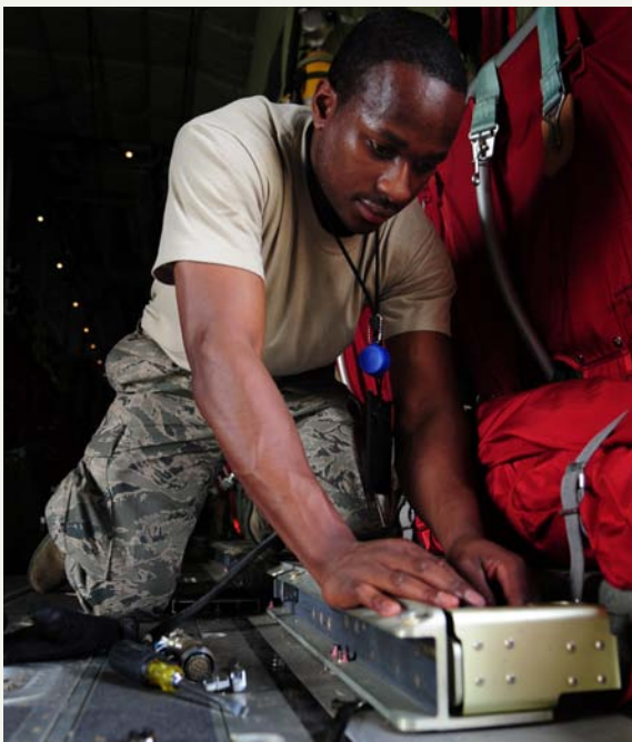
Left: U.S. Air Force Senior Airman Travis Dale, 86 Aircraft Maintenance Squadron crew chief, affixes a personnel jump platform to the side door of a C-130J in preparation of Romanian Air Force members for a jump during the joint exercise Carpathian Summer, Airlift Base Otopeni, Romania, May 10, 2010. (U.S. Air Force Photo by Staff Sgt. Jocelyn Rich)
