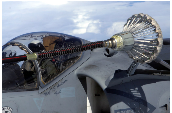
An AV-8B Harrier pilot with Marine Attack Squadron 223, Marine Aircraft Group 14, 2nd Marine Aircraft Wing, currently attached to the 31st Marine Expeditionary Unit air combat element, inserts his jet's probe into a drogue, a stabilization device fitted on a KC-130J Hercules' refueling hose, during a mission with Marine Aerial Refueler Transport Squadron 152, MAG-36, 1st MAW, Oct. 8. (Photo by Lance Cpl. Stefanie C. Pupkiewicz)
