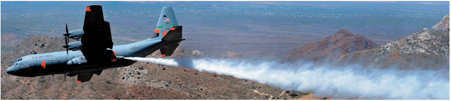
C-130Js equipped with MAFFS systems and loaded with thousands of pounds of water took to the Arizona skies for training this month. Photo by John Rossino.
