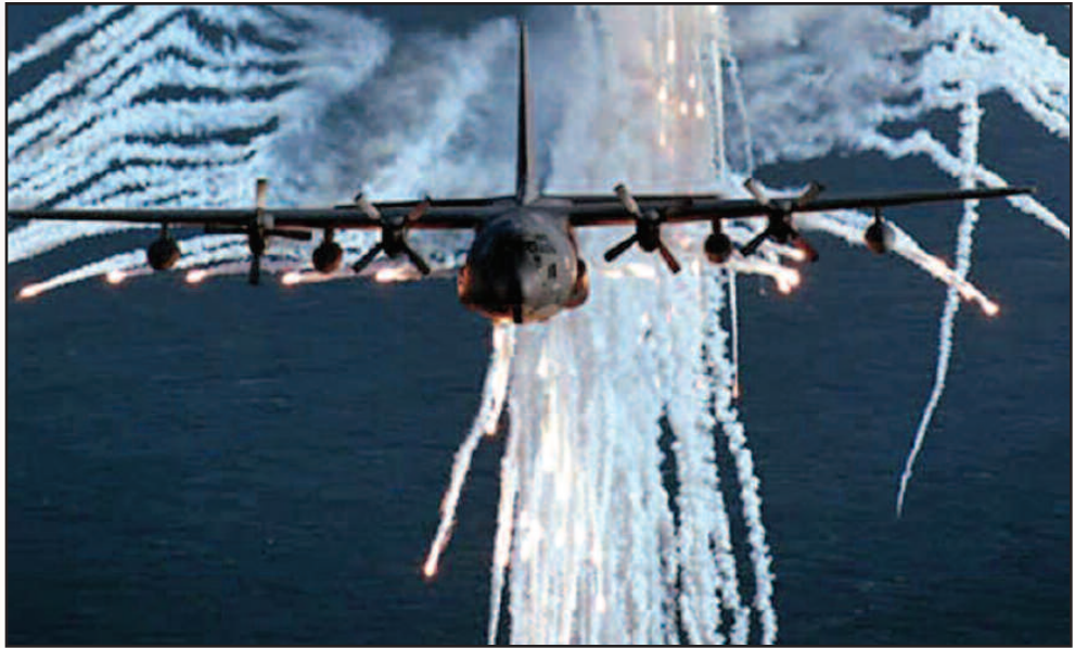
The C-130 can be equipped with extensive self-protection features such as the flares being dispensed in this picture that distract heat-seeking missiles from the aircraft.
