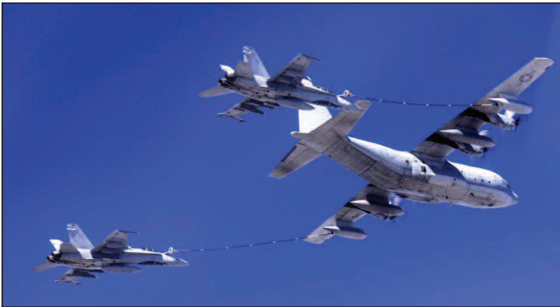
The KC-130 aerial refueling tanker enables aircraft such as these two Navy fighters to refuel in flight, extending their range and flexibility in combat operations.
